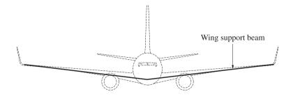
Assume the engines are supported by the single beam. The beam runs through the plane, wing tip to wing tip.
