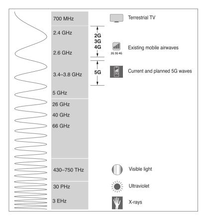
With reference to the diagram, explain why 5G networks need more cellular antennae and closer positioning of antennae than 4G networks. (3 marks)
